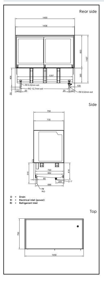
Drop-In Drop-in remote refrigerated well with refrigerated display, squared, medium service - 4 hours - 4GN The company reserves the right to make modifications to the products without prior notice. All information correct at time of printing.
