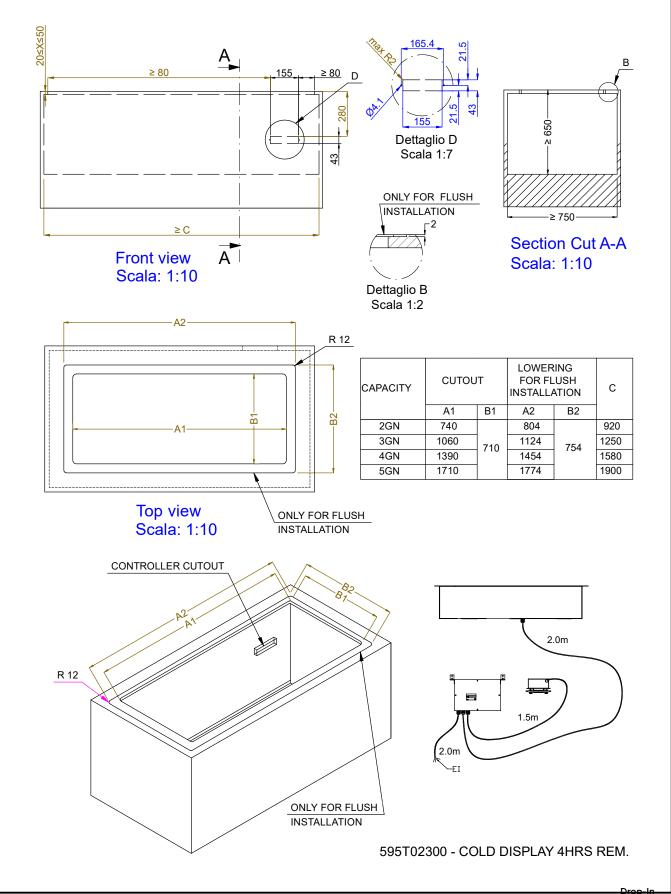
Drop-in Drop-in remote refrigerated well with refrigerated display, squared, medium service - 4 hours - 4GN The company reserves the right to make modifications to the products without prior notice. All information correct at time of printing.
